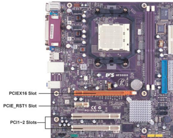
**PCIEX16 Slot** The PCI Express x16 slot is used to install an external PCI Express graphics card that is fully compliant to the PCI Express Base Specification revision 1.0a.
