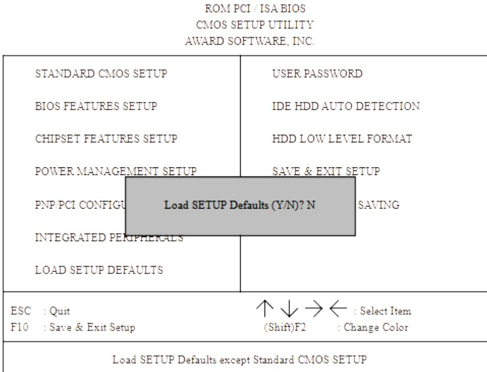
Figure 4.7: Load Setup Defaults
