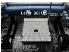
STEP 1: Lift Up The Socket Lever
