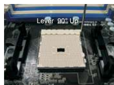
STEP 1: Lift Up The Socket Lever
