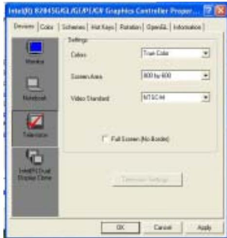
If you connect the Monitor and LCD panel at the same time, here can let you configure if you want to have a clone dual display function. (Notice: TV-out does not have the ability with dual display.)
