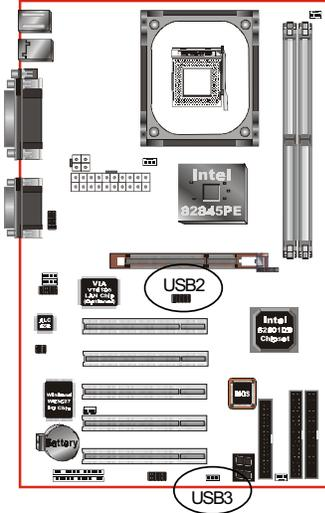
**USB2/3:** USB port header for four USB2.0 ports. It will help your device more efficient for the transfer speed up to 480Mbps.
