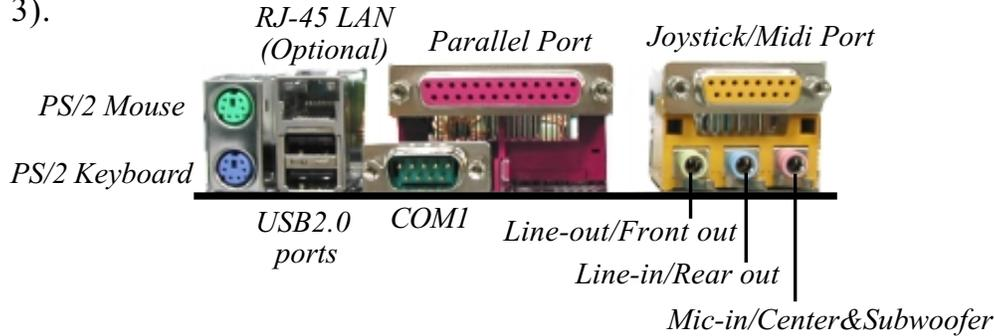
Figure 3: I/O back panel layout
