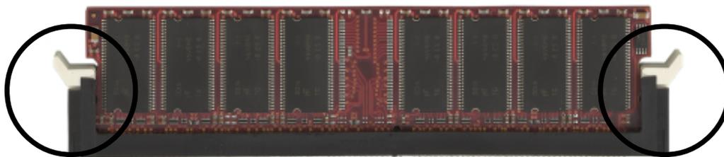
*Figure 10 - DIMM module clip after installation*
