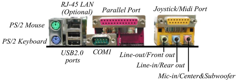
Figure 11 - I/O Ports
