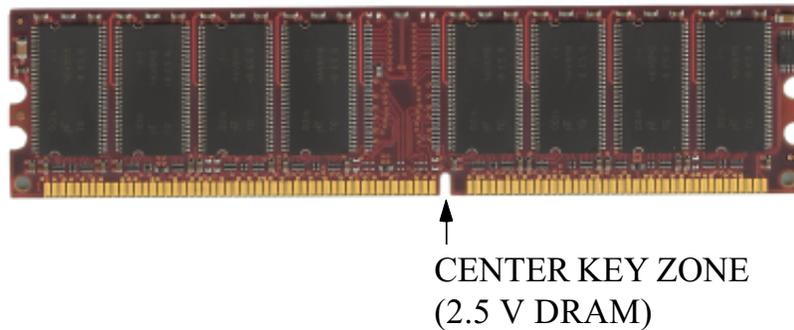
*Figure 8 - DIMM notch*
