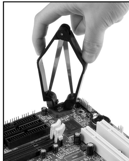
The BIOS socket may be damaged if using an improper method to replace the BIOS chip.
