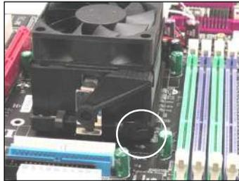
6. Locate the Fix Lever, Safety Hook and the Fixed Bolt.
