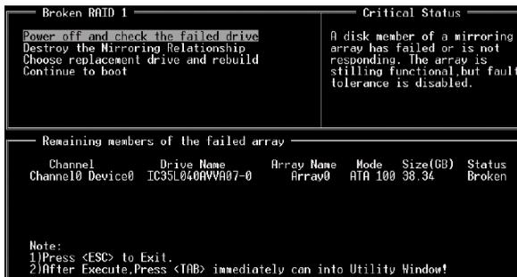
**1. Power off and Check the Failed Drive:**
