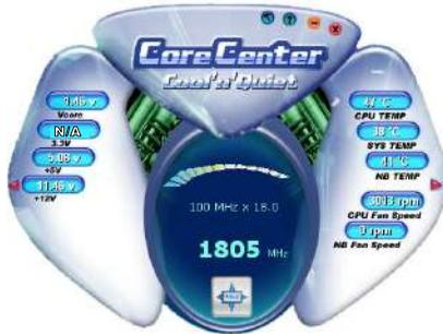
Here the current system status (including Vcore, 3.3V, +5V and 12V) and the current PC hardware status (such as the CPU & system temperatures and all fans speeds) are shown on the left and right sides for you to monitor.
