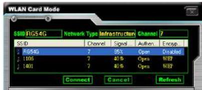
If the network you are selecting is encrypted (**WEP** shown in the **Encryption** column), the screen will display as below. You need to enter the correct WEP key defined by AP in the specified **WEP Key 1~4** fields to make the connection.
