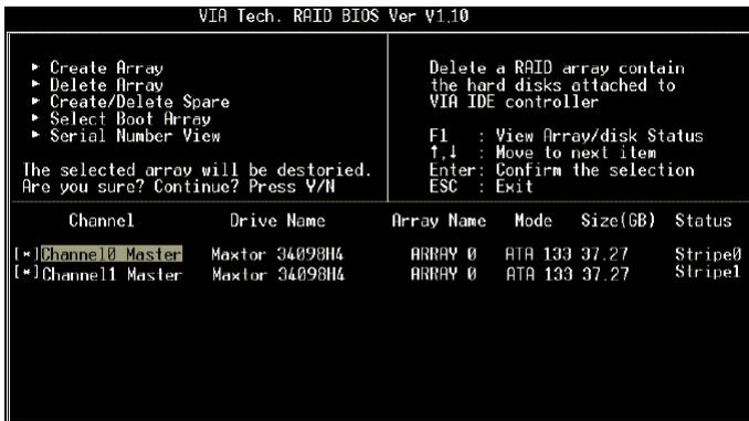
Deleting a disk array will destroy all the data on the disk array except RAID 1 arrays. When a RAID is deleted, the data on these two hard disk drives will be reserved and become two normal disk drives.
