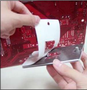
2. Turn over the mainboard, and install the backplate to the proper position.
