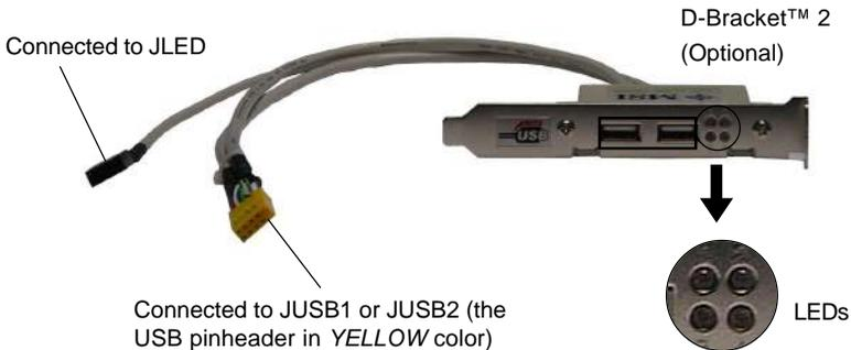
D-Bracket™ 2 is an external USB bracket integrating four Diagnostic LEDs, which use graphic signal display to help users understand their system. The LEDs provide up to 16 combinations of signals to debug the system. The 4 LEDs can debug all problems that fail the system, such as VGA, RAM or other failures. This special feature is very useful for the overclocking users. These users can use the feature to detect if there are any problems or failures.
