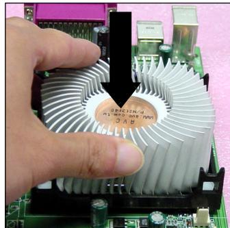
3. Mount the fan on top of the heatsink. Press down the fan until its four clips get wedged in the holes of the retention mechanism.
