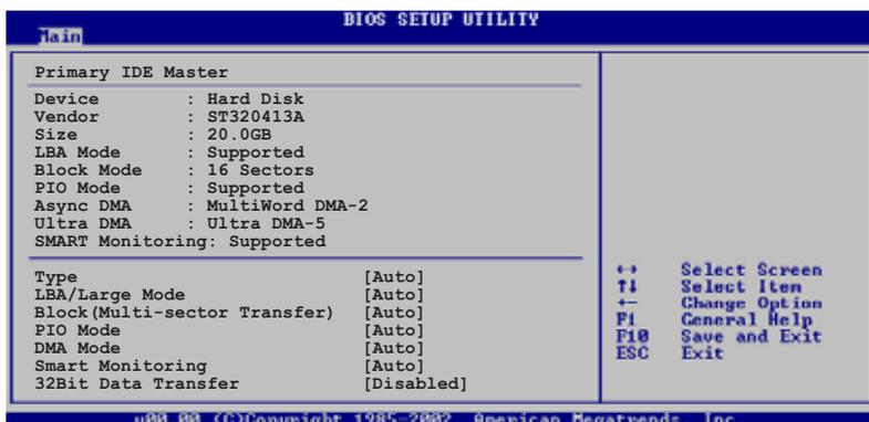
The BIOS automatically detects the values opposite the dimmed items (Device, Vendor, Size, LBA Mode, Block Mode, PIO Mode, Async DMA, Ultra DMA, and SMART monitoring). These values are not user-configurable. These items show N/A if no IDE device is installed in the system.
