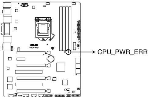
**P9D WS CPU\_PWR\_ERR LED**
