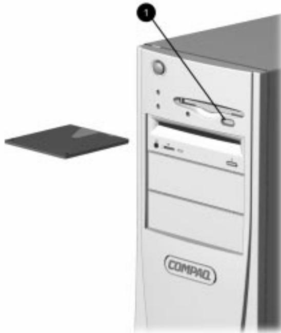
*Manually Removing a Diskette from the LS-120 Drive*
