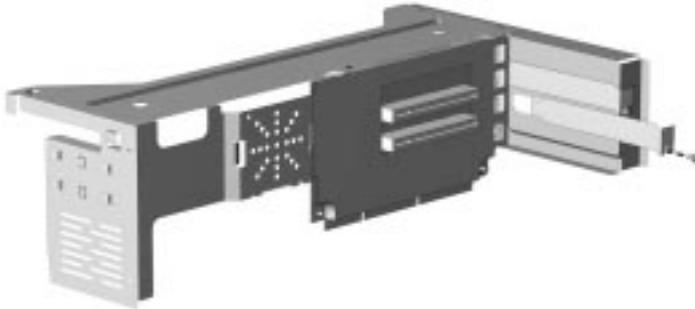
**Removing the Screw and Expansion Slot Cover**
