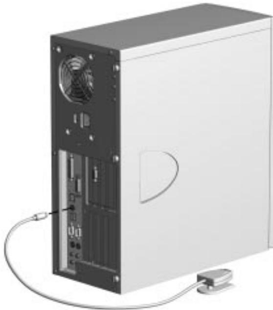
*Connecting an External Infrared Transceiver*
