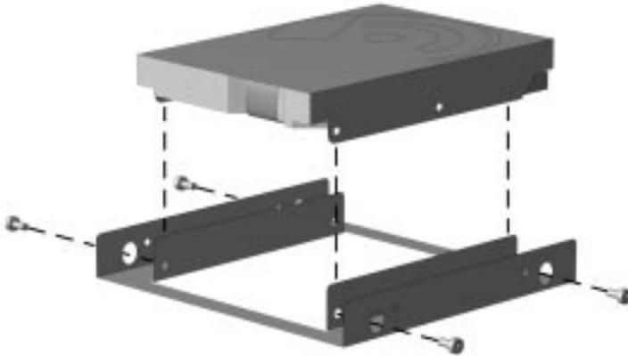
*Attaching a 3.5-Inch Drive to the 5.25-Inch Bracket*
