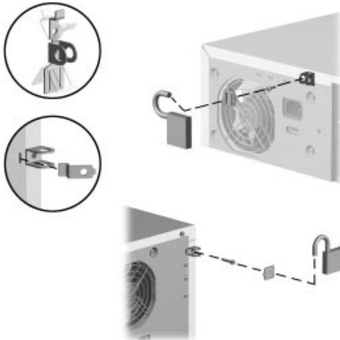
*Attaching a Security Bracket with Padlock*
