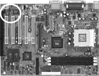
This connector is for Surround and Center+Bass speaker output ext. Plug in the optional AC3 Surround/Center+Bass jack extension into this connector. The black colored jack is for surround speaker output and the orange colored jack is for center+bass speaker output.
