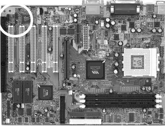
The S/PDIF-out connector supports the digital audio. This connector must be connected to the cable from an external device (i.e.2-channel decoded AC-3 from DVD decoders).
