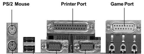
PS/2 Mouse      Keyboard      USB 1/2      COM1      COM2      Line-out      Line-in      MIC
