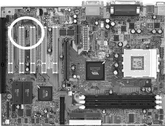
If you enable the UART 2 Mode in BIOS's Integrated Peripherals menu the COM2 port will support IR functions. (See section 3-4)
