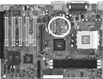
This connector is to be connected to an optional TV/LCD/2nd CRT Output adapter card.
