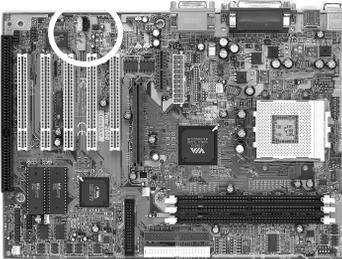
Use the audio cable enclosed with your CD-ROM disk drive to connect the CD-ROM to your mainboard. This will enable your CD-ROM's audio function.
