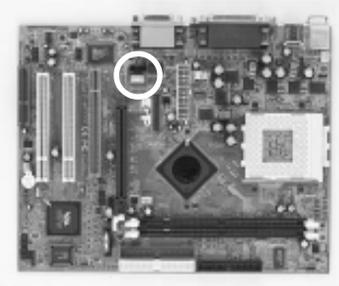
Use the auxiliary audio cable enclosed with your CD-ROM disk drive to connect the CD-ROM to your mainboard. This will enable your CD-ROM's audio function.
