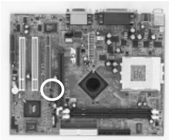
This feature allows you to enable and disable the USB function on ACR slot. You must set the jumper's cap to pins 1-2 and 3-4 to enable this function. Leave jumper's pin 1-2 and 3-4 open to disable this function
