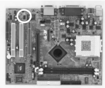
This connector is for Center+Bass speaker output ext. Plug in the optional AC3 Surround Center/Bass and Rear left/right jack extension into this connector. The black colored jack is for surround speaker output and the orange colored jack is for center+bass speaker output.
