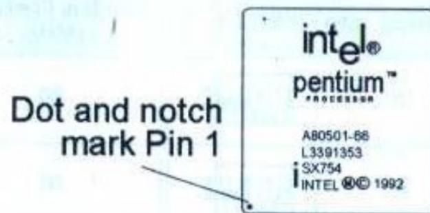
Figure 2-1 The markings on top of a CPU
