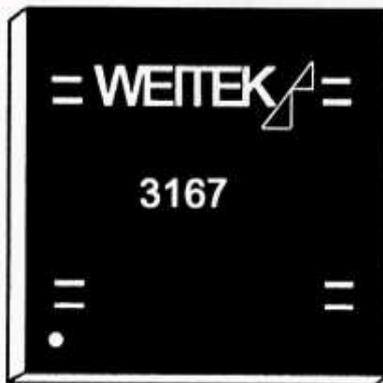
The numeric coprocessor socket on the 333UC/340UC/333UCB/340UCB system board is designed for a 25, 33 or 40 MHz Intel 80387, or compatible, coprocessor, such as a Cyrix, ULSI, or Weitek 3167.
