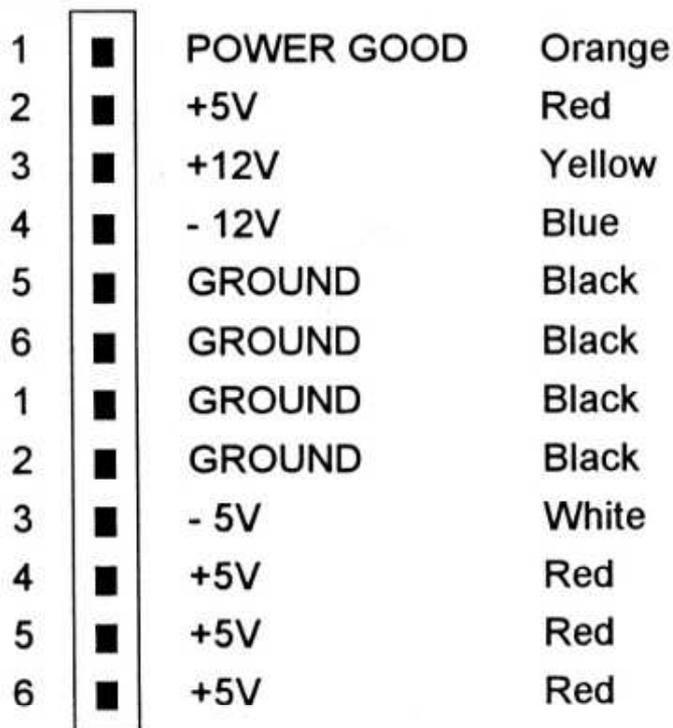
Figure3-2 Power Supply Connector
