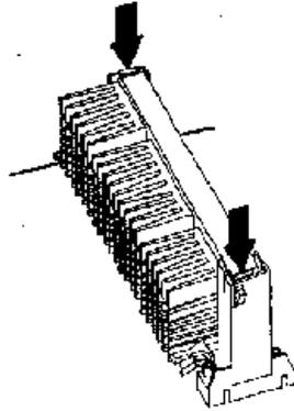
Hook the top support of the heat sink to the support base of the heat sink to complete the CPU module installation:
