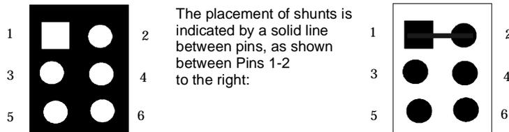
**CPW Clear Password** CPW is a 2-pin berg that allows you to delete the system BIOS password should you forget the password. CPW should be OPEN at all times during normal operation. Should you forget the password: turn power off, remove the computer cover, turn power on, place a shorting bridge (shunt) on CPW for a few seconds, then turn power off again. Reboot the computer and re-enter all system configuration information, because you have just erased all of it.
