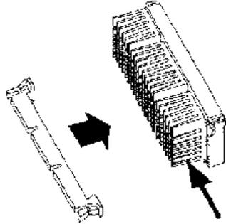
The slide the CPU module into the Retention Mechanism Assembly, as shown below:
