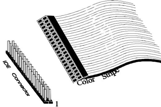
PRIMARY is a 40-pin dual-inline berg that connects an IDE drive to the primary onboard IDE connector. This motherboard supports IDE Modes 0, 1, 2, 3, and 4, IDE prefetch, LBA (Logical Block Address) mode, high capacity drives (over 528 MB), 32-bit data transfer, and fast IDE transfer. These IDE features are configured in Peripheral Setup in the AMIBIOS Setup utility. Disable the onboard IDE interface in Peripheral Setup to use an ISA ESDI, RLL, MFM, or SCSI hard disk drive controller.
