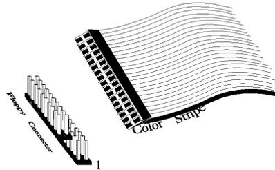
The motherboard supports up to two 720 KB, 1.44 MB, or 2.88 MB 3½" drives and 360 KB and 1.2 MB 5¼" drives. The connecting cable is a 34-pin ribbon connector with two 34-pin edge connectors for attaching the floppy disk drives. There is a small twist in the cable between the floppy connectors. The last (end) connector should be connected to floppy drive A:.
