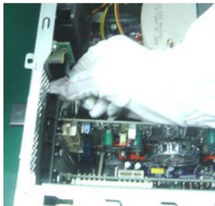
2. Release the VGA-slot Lock shown bellow, then pull out the VGA Card.
