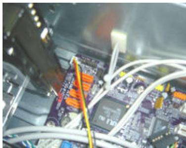
11. Disconnect the ODD&FDD IDE and P1 power cable from the M/B connector.
