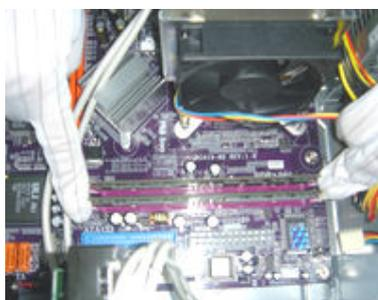
Remove the Heatsink module.
