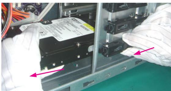
3. Release the FDD-Holder, meanwhile pull the Card-reader Module out of the chassis.
