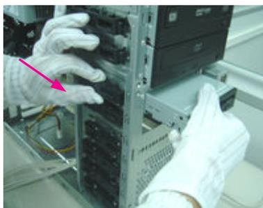
Release the ODD-Holder, meanwhile pull the Slave ODD out of the chassis, then the Master one.
