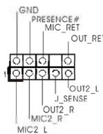
This header is for connecting audio devices to the front audio panel.
