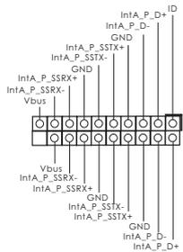
Besides two USB 3.0 ports on the I/O panel, there is one header on this motherboard. This USB 3.0 header can support two ports.
