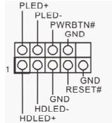
Connect the power switch, reset switch and system status indicator on the chassis to this header according to the pin assignments below. Note the positive and negative pins before connecting the cables.
