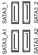
These four SATA3 connectors support SATA data cables for internal storage devices with up to 6.0 Gb/s data transfer rate.
