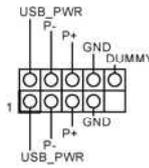
Besides two USB 2.0 ports on the I/O panel, there are two headers on this motherboard. Each USB 2.0 header can support two ports.
