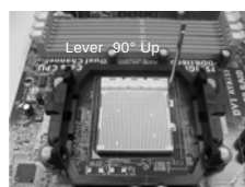
STEP 1: Lift Up The Socket Lever
