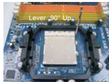
STEP 1: Lift Up The Socket Lever
