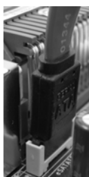
Connect the SATA data cable to the eSATAII connector (eSATAII_TOP)
