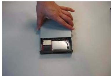
11. Remove the two screws on each side of HDD and then detach the HDD holder.
