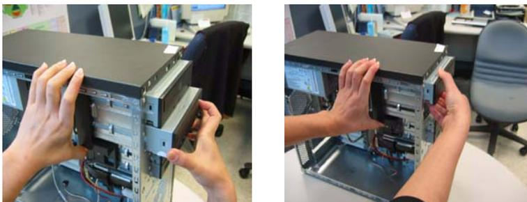
7. Press the FDD lock upward and detach the FDD from the frame.
