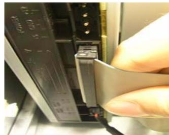
3. Disconnect the ODD2 power cable and ODD2 cable from the ODD.
