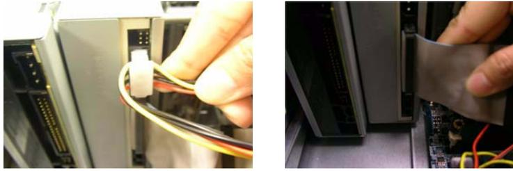
4. Disconnect the FDD power cable and the FDD cable from the FDD.
