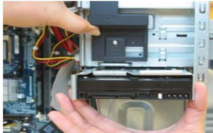
10. Remove the two screws on each side of Card Reader and then detach the Card Reader holder.
