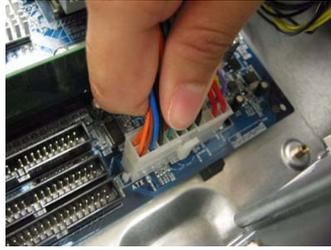
2. Remove the ATX-12V power connector as shown here.
