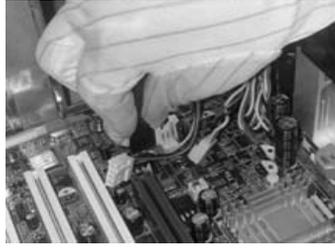
2. Disconnect the FDD cable from the mainboard.
