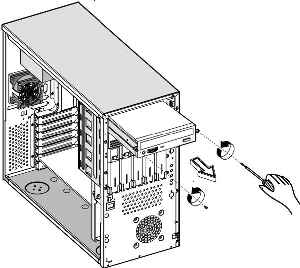
4. Remove the rails from the old drive by removing four screws. Keep the screws for later use.
