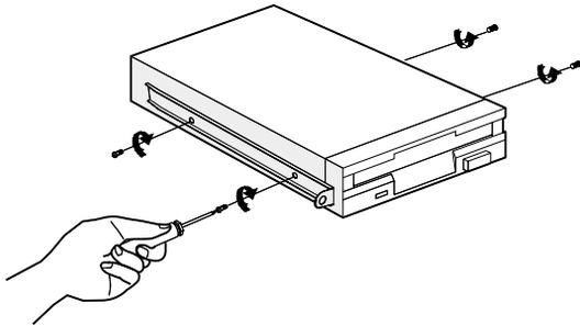
6. Insert the new drive into the drive bay and secure it with the two screws removed in step 3.
