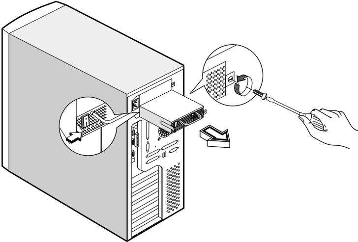
3. Gently pull the power supply module out.
