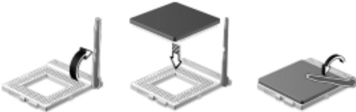
3. Attach one side of the fan/heatsink metal bracket to the CPU socket and then gently push the other side of the metal bracket down until it locks in place.
