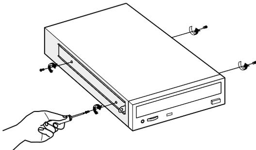
6. Insert the new drive into the drive bay and secure it with two screws.
