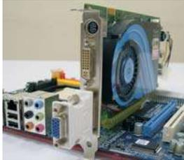
Step 7. Install the other Radeon graphics card to PCIE3 slot. For the proper installation procedures, please refer to section "Expansion Slots".
