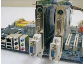
Step 8. Connect two Radeon graphics cards by installing two CrossFire™ Bridge on CrossFire™ Bridge Interconnects on the top of Radeon graphics cards. (CrossFire™ Bridge is provided with the graphics card you purchase, not bundled with this motherboard. Please refer to your graphics card vendor for details.)
