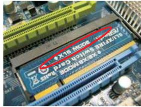
Step 3. To change it to CrossFire Mode, you need to reverse the direction of ASRock SLI/XFire Switch Card. Please simultaneously pull open both the retention arms that hold the card in position. The card itself will spring away from the retention slot. Take it out gently by holding its edges, and keep away from touching the connectors (Golden Fingers).
