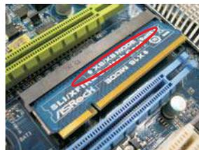
Step 5. Push the card down into the retention slot till both the retention arms firmly hold the card into position. Also, keep away from touching the connectors (Golden Fingers).
