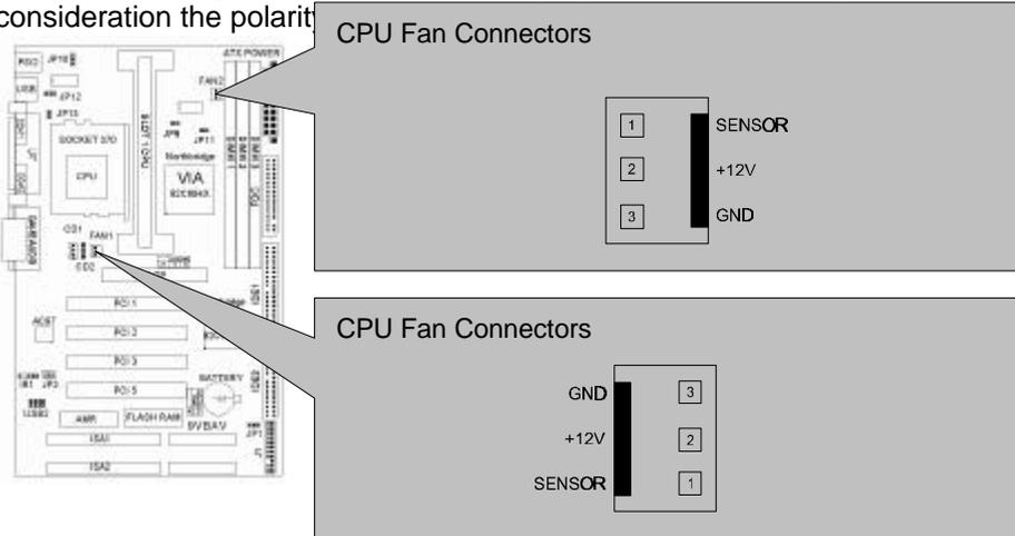
Note: The CPU and motherboard will overheat if there is no airflow across the CPU and onboard heatsink. Damage may occur to the motherboard and the CPU fan if these pins are incorrectly used. These are not jumpers, do not place jumper caps over these pins.
