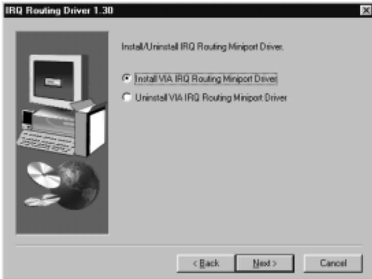
10. The driver files will now be installed. When finished installing, choose the "Yes" to reboot option and click "Finish" to restart your computer. The driver should now be loaded.
