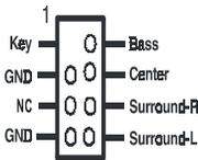
This connector is for Surround and Center+Bass speaker output ext. Plug in the optional AC3 Surround/Center+Bass jack extension into this connector. The black colored jack is for surround speaker output and the orange colored jack is for center+bass speaker output.
