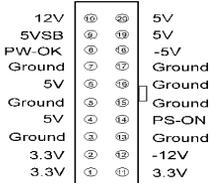
The ATX power supply provides a single 20-pin connector interface which incorporates standard +/-5V, +/-12V, optional 3.3V and Soft-power signals. The Soft-power signal, a 5V trickle supply is continuously supplied when AC power is available. When the system is in the Soft-Off mode, this trickle supply maintains the system in its minimum power state.
