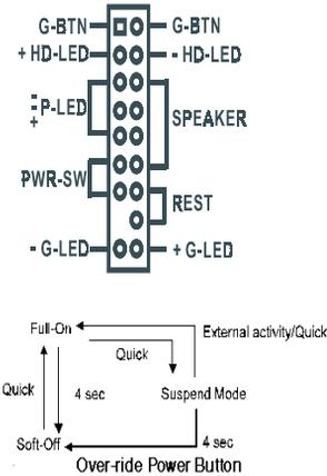
The power button on the ATX chassis can be used as a normal power switch as well as a device to activate Advanced Power Management Suspend mode. This mode is used for saving electricity when the computer is not in use for long periods of time. The Soft-OFF by PWR-BTTN function in BIOS's Power Management Setup menu must be set to "Delay 4 Sec." to activate this function.
