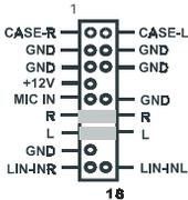
This connector give you the option of a front panel audio jack cable ext. to be plug into a special custom designed system case. Simply remove the two jumper caps at pin 11-12 and 13-14 then plug it into the (optional) cable ext. connector. Pin 11-12 and 13-14 are shorted (default) to enabled the back panel audio function.
