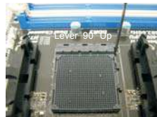
STEP 1: Lift Up The Socket Lever
