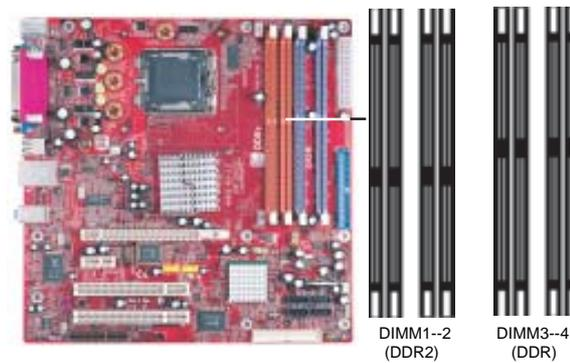
**Note1:** Please be noted you can **NOT** use DIMM1-2(DDR2 533/DDR400) and DIMM3-4(DDR400) simultaneously. Only use either DDR2(533/400) or DDR(400) memory modules!
