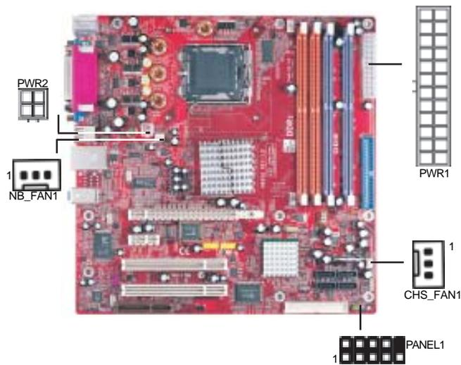
Connect the power connector from the power supply to the **PWR1** connector on the motherboard. The **PWR2** is a +12V connector for CPU Vcore power.
