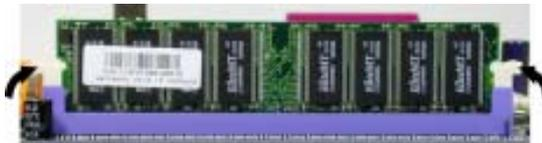
4. Install any remaining DIMM modules.
