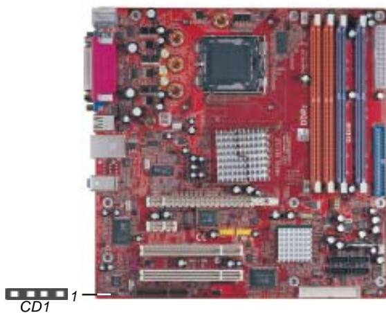
When you first start up your system, the BIOS should automatically detect your CD-ROM/DVD drive. If it doesn't, enter the Setup Utility and configure the CD-ROM/DVD drive that you have installed. On the motherboard, locate the 4-pin header **CD1**.
