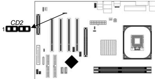
When you first start up your system, the BIOS should automatically detect your CD-ROM/DVD drive. If it doesn't, enter the Setup Utility and configure the CD-ROM/DVD drive that you have installed. On the motherboard, locate the 4-pin connector **CD2**.
