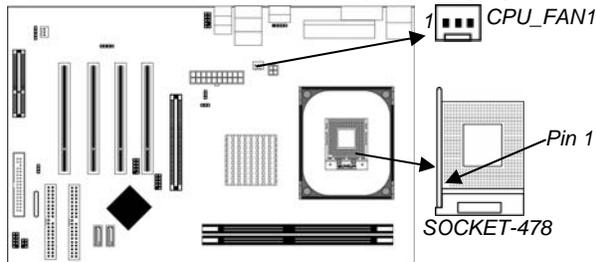
1. Unhook the locking lever of the CPU socket. Pull the locking lever away from the socket and raising it to the upright position.
