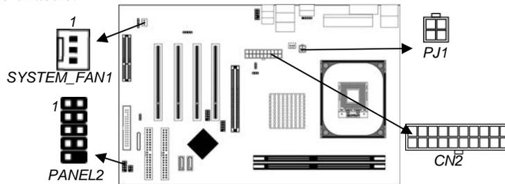
Connect the power connector from the power supply to the **CN2** connector on the motherboard. The **PJ1** is a +12V connector for CPU Vcore power.
