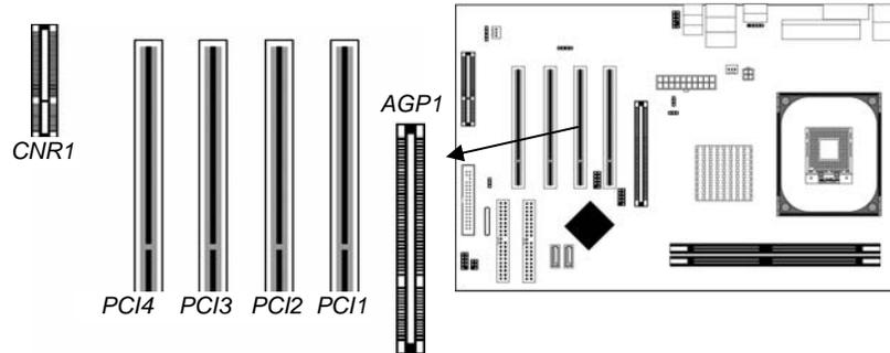
Follow the steps below to install an AGP/CNR/PCI expansion card.
