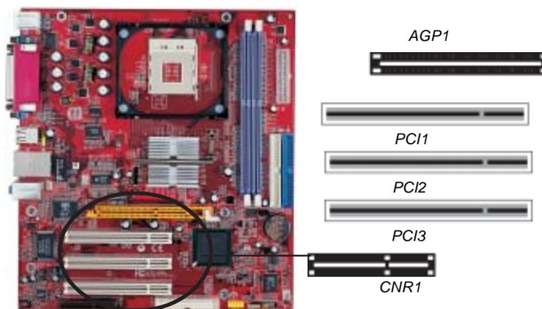
Follow the steps below to install a CNR/PCI expansion card.
