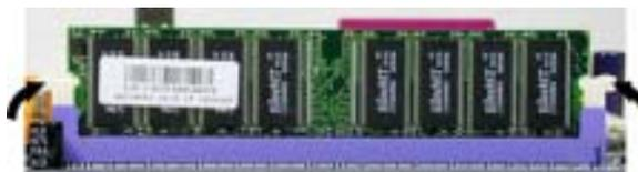
4. Install any remaining DIMM modules.
