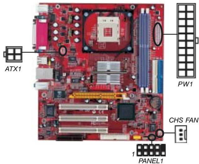
Connect the power connector from the power supply to the **PW1** connector on the motherboard. The **ATX1** is a +12V connector for CPU Vcore power.
