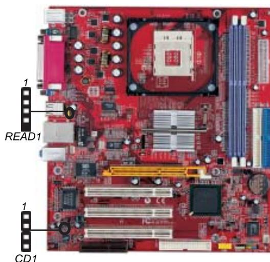
When you first start up your system, the BIOS should automatically detect your CD-ROM/DVD drive. If it doesn't, enter the Setup Utility and configure the CD-ROM/DVD drive that you have installed. On the motherboard, locate the 4-pin header **CD1**.
