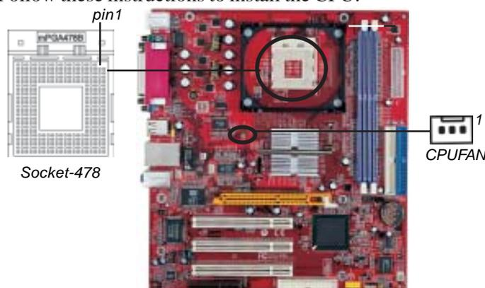
1. Unhook the locking lever of the CPU socket. Pull the locking lever away from the socket and raising it to the upright position.
