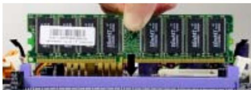
3. Install the DIMM module into the socket and press it firmly down until it is seated correctly. The socket latches are levered upwards and latch on to the edges of the DIMM.
