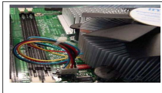
9. Secure excess cable with tie-wrap to ensure cable does not interfere with fan operation or contact other components.
