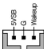
Enable the Wake Up On Modem selection in BIOS's Power Management Menu to activate this function. This header is used to connect an add-in modem card, which gives WOM capability to the motherboard.
