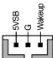
Enable the Wake Up On LAN selection in BIOS's Power Management Menu to use this function. The capability to remotely manage PCs on a network is a significant factor in reducing administrative and ownership costs. Magic Packet technology is designed to give WOL capability to LAN controller. This header is used to connect an add-in NIC (Network Interface Card) that gives WOL function to the motherboard.
