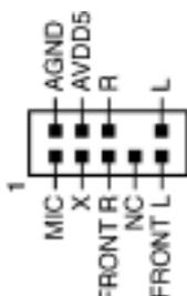
This connector gives you the option of a front-panel audio jack cable ext. to be plugged into a special custom-designed system case. Simply remove the two jumper caps at pin [5-6] and [9-10] then plug it into the (optional) cable ext. connector. Pin [5-6] and [9-10] are shorted (default) to enable the back-panel audio function.
