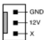
The board's hardware management is able to detect the CPU and system fan speed in rpm (revolutions per minute). The wiring and plugging may vary depending on the manufacturer. On standard fans, the red is positive (+12V) and the black is ground.
