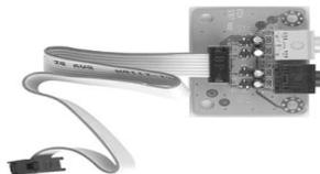
Figure 1-4 (Optional) 6 Channel Audio Adapter card
