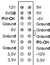
The power cord leading from the system's power supply to the external power source must be the very last part connected when assembling a system. The ATX power supply provides a single 20-pin connector interface which incorporates standard +/-5V, +/-12V, optional 3.3V and Soft-power signals. The Soft-power signal, a 5V trickle supply is continuously supplied when AC power is available. When the system is in the Soft-Off mode, this trickle supply maintains the system in it's minimum power state.
