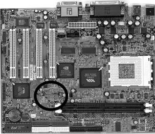
This connector is to be connected to an optional LCD/TV-out adapter card.
