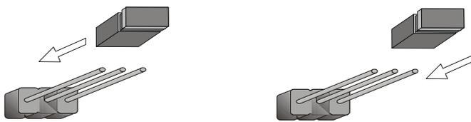
**Normal(1-2 closed)    Reset CMOS(2-3 closed)**
