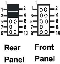
This connector give you the option to choose between standard audio jack(rear panel) or use a an optional front panel audio jack cable ext. to be plug into a special custom designed system case. To use the standard audio jack short jumper caps to pin 1-2 and pin 3-4 (Default). To use the front panel audio jack cable ext., simply removed both jumper caps and plug into the audio jack cable.
