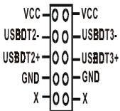
If you want to use a USB Keyboard, you must enable the USB keyboard support function in BIOS's Integrated Peripherals menu (See Section 3-4). This board contains a USB Host controller and includes a root hub with two USB 1/2 ports a connector for optional USB Adaptor (USB 3/4).
