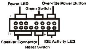
The power button on the ATX chassis can be used as a normal power switch as well as a device to activate Advanced Power Management Suspend mode. This mode is used for saving electricity when the computer is not in use for long periods of time. The Soft-OFF by PWR-BTTN function in BIOS's Power Management Setup menu must be set to "Delay 4 Sec." to activate this function.
