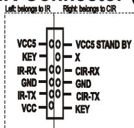
Select a UART Mode in BIOS's Integrated Peripherals menu the UART port to support IR/CIR functions. (See section 3-4)
