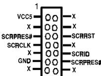
This connector must be connected to a Smart card reader .
