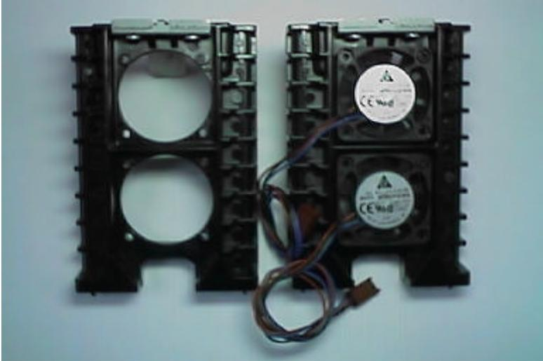
Figure 1: Dual Processor Retention Mechanism
