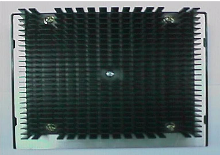
Figure 4:Boxed Pentium® II/ III XEON SLOT2 Processor & Heat sink support
