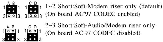
Short pin 1-2 to enable Soft Modem riser only (On-board AC97 CODEC enabled). Short pin 2-3 to enable Soft Audio Modem riser (On-board AC97 CODEC disabled).
