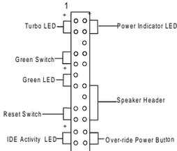
When the Soft-OFF by PWR-BTTN function is enabled, pushing the power button rapidly will switch the system to Suspend mode. Any occurrence of external activities such as pressing a key on the keyboard or moving the mouse will bring the system back to Full-On. Pushing the button while in Full-On mode for more than 4 seconds will switch the system completely off. See Over-ride Power Button Operation diagram.
