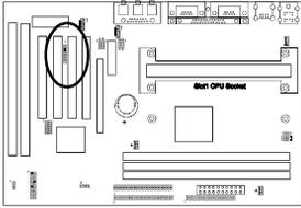
If you enable the COM2 Mode in BIOS's Integrated Peripherals menu the COM2 port will support IR functions. (See section 3-8)
