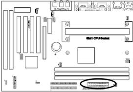
This mainboard requires a power supply of at least 200 watts. The power cord leading from the system's power supply to the external power source must be the very last part connected when assembling a system.
