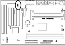
Use the audio cable enclosed with your CD-ROM disk drive to connect the CD-ROM to your mainboard. This will enable your CD-ROM's audio function.
