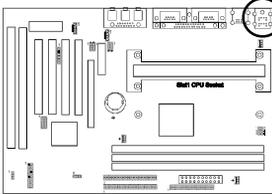
If a PS/2 mouse is used, BIOS will automatically detect and assign IRQ12 to the PS/2 mouse.
