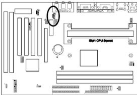
Use the cable enclosed with your CD-ROM disk drive to connect the CD-ROM to your mainboard. This will enable your CD-ROM's audio function.
