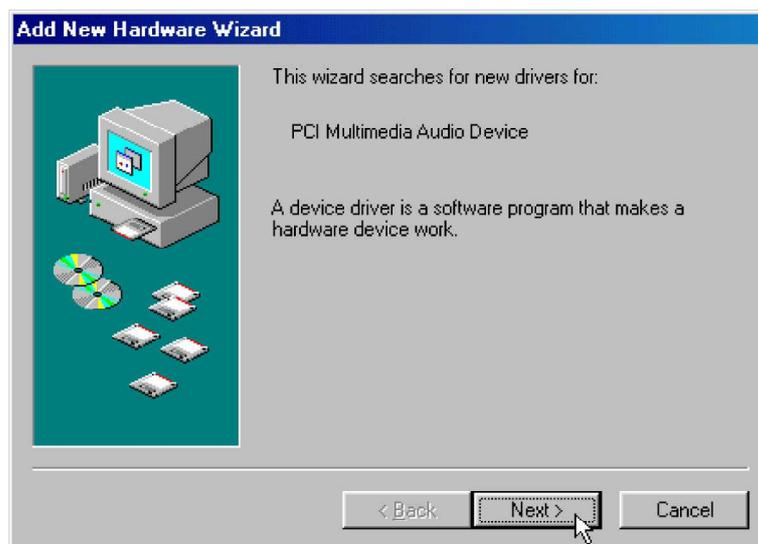
2. As Windows95/98 starts up, it will automatically detect the audio controller and start the driver installation. Windows95/98 will detect the audio controller as "**PCI Multi media Audio Device**". The Wizard will guide you to begin the driver installation.
