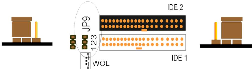
The default Power On function is “Button Only”. That means, we can only turn our computer on and off by pressing the “Power Button”. If we want to enable KB & PS/2 Mouse Power On function, we first have to set JP9 Pin 1-2 closed, and then go to “Power On Function” in “Integrated Peripherals” of Award BIOS Setup. At the line “Power On Function”, we can press “Page Up” or Page Down” to make one of the following selections:
