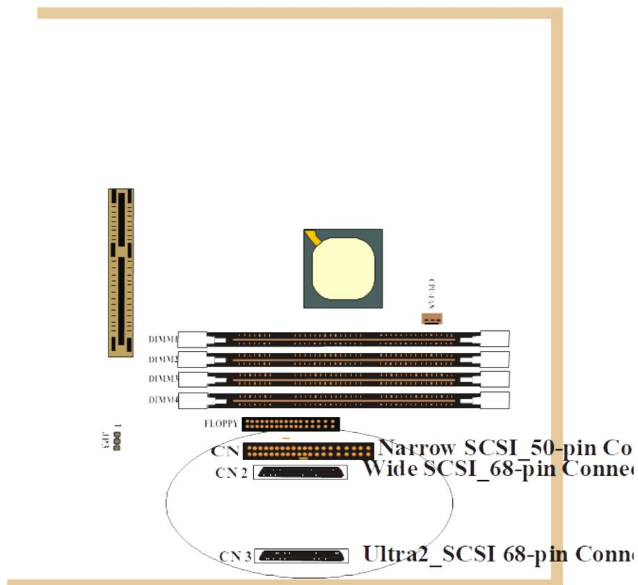
**6258M Mainboard** is built in with SCSI BIOS supported by Adaptec SCSI Chipset AIC-7890 and AIC-3860.
