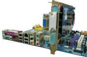
Step 3. Install the other Radeon graphics card to AGI Express slot (PCI Express x4). For the proper installation procedures, please refer to section “Expansion Slots”.
