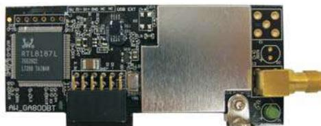
ASRock WiFi-802.11g module is an easy-to-use wireless local area network (WLAN) adapter to support WiFi+AP function. With ASRock WiFi-802.11g module, you can easily create a wireless environment and enjoy the convenience of wireless network connectivity. Therefore, from anywhere within the signal range, you will be able to play LAN games, connect to the internet, access and share printers, and make Internet phone calls easily.
