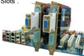
Step 4. Connect two Radeon graphics cards by installing two CrossFire™ Bridge Interconnects on the CrossFire™ Bridge Interconnects on the top of Radeon graphics cards. (CrossFire™ Bridge is provided with the graphics card you purchase, not bundled with this motherboard. Please refer to your graphics card vendor for details.)
