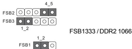
Note3: If you use a FSB1066-CPU and adopt a DDR2 1066 memory module on this motherboard, you need to adjust the jumpers. Please short pin2, pin3 for FSB3. Otherwise, the CPU and memory module may not work properly on this motherboard. Please refer to below jumper settings.
