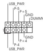
Besides four default USB 2.0 ports on the I/O panel, there are three USB 2.0 headers on this motherboard. Each USB 2.0 header can support two USB 2.0 ports.
