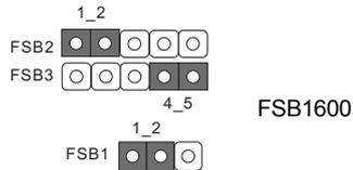
Note2: If you use a FSB1333-CPU and adopt a DDR2 1066 memory module on this motherboard, you need to adjust the jumpers. Please short pin4, pin5 for FSB2. Otherwise, the CPU and memory module may not work properly on this motherboard. Please refer to below jumper settings.
