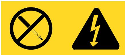
Hazardous voltage, current, and energy levels are present inside any component that has this label attached. There are no serviceable parts inside these components.
