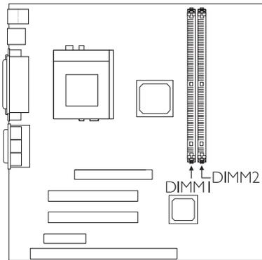
The system board also supports the ECC (Error Checking and Correction) function. To use this function, you must install DIMM that supports parity. Refer to chapter 1 (System Memory section) for detailed specification of the memory supported by the system board.
