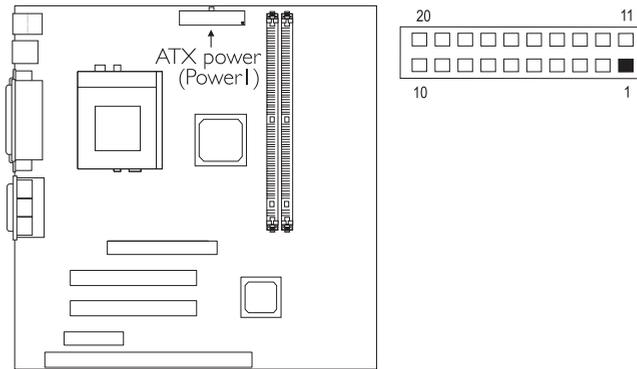
The pin assignment of the ATX power connector is shown below.
