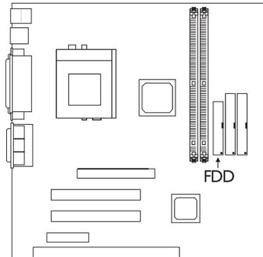
2. Install the other 34-pin header connector(s) into the disk drive(s). Align the colored edge of the daisy chained ribbon cable with pin 1 of the drive edge connector(s). The end-most connector should be attached to the drive you want to designate as Drive A.
