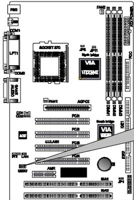
**Universal Serial BUS (USB) PIN Header**
