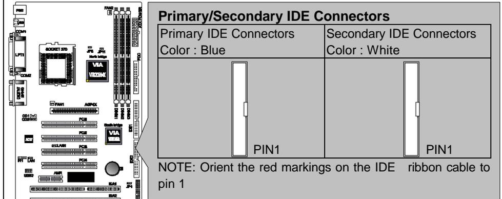
Note: Ultra DMA/66 IDE devices must use an 80-wire IDE cable or else devices will automatically be limited to Ultra DMA/33 mode.
