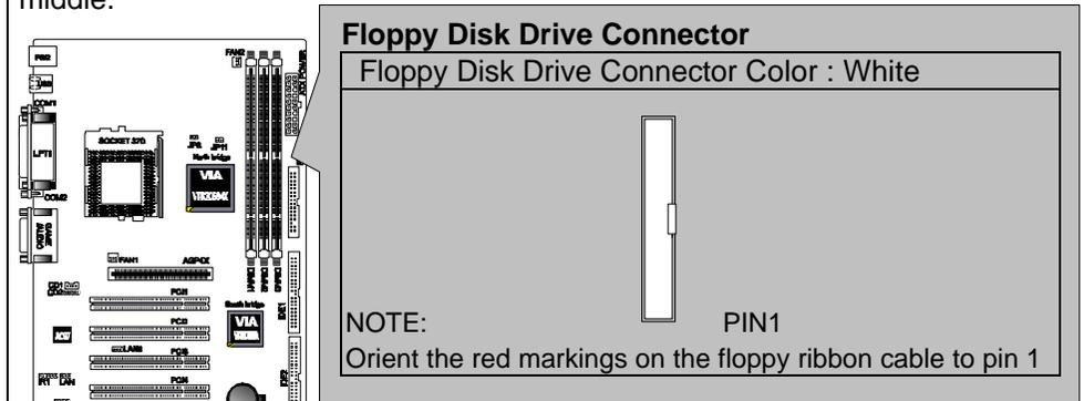
Note: Pin 5 is removed to prevent the users inserting the Floppy Disk Drive in the wrong orientation when using ribbon cables with pin 5 plugged.
