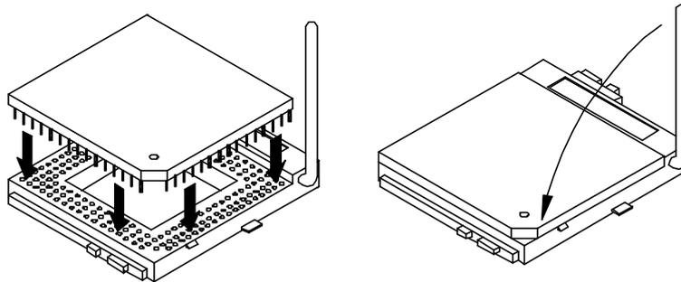
After you have installed the processor into socket, check if the jumpers for the CPU type and speed are correct.
