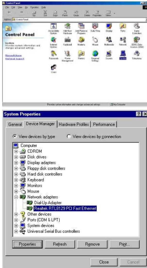
2. Under System Properties, click on the Device Manager tab. Double click on Realtek 8129 PCI Fast Ethernet. Click the Driver tab as shown. Now click the Update Driver button.
