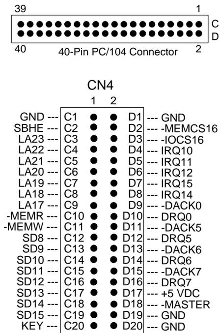
Figure 3-10 CN4: 40-Pin PC/104 Connector Bus C & D
