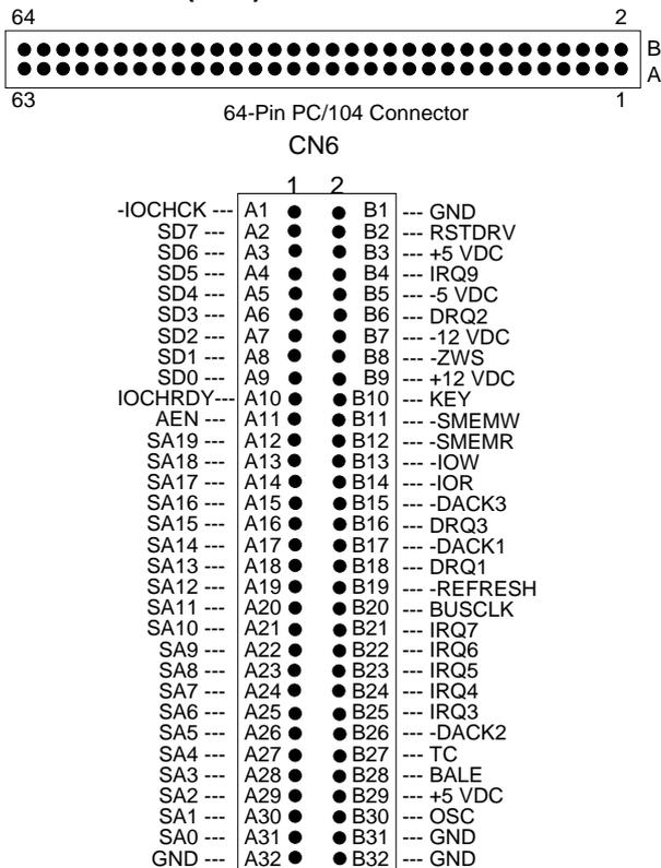
Figure 3-9 CN6: 64-Pin PC/104 Connector Bus A & B
