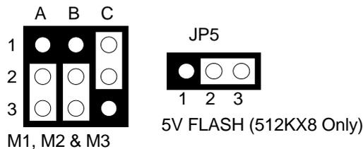
Figure 5-8 Large Page 5V FLASH Jumper Setting
