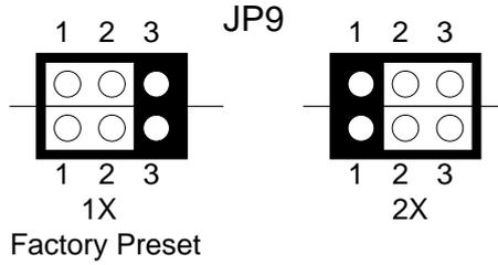
**Figure 3-14 JP9: CPU System Clock Multiplier Select**
