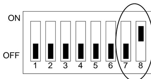
Figure 5-9 5V FLASH (29CXXX & 28EEXXX) Switch Setting
