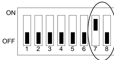
Figure 5-7 5V Large FLASH (29FXXX) Switch Setting
