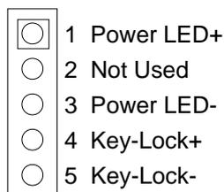
Figure 3-16 J4: Power LED & Key Lock Header
