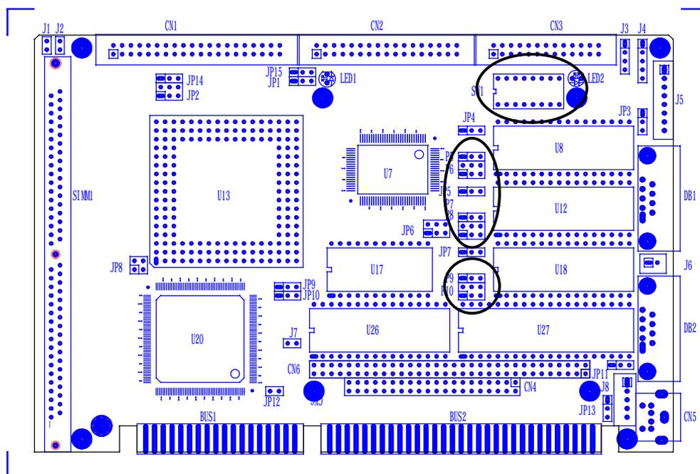
Figure 5-1 Switch & SSD Type Jumper Location
