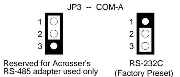
**Figure 3-2 JP3: RS-485 Adapter Select for COM-A**
