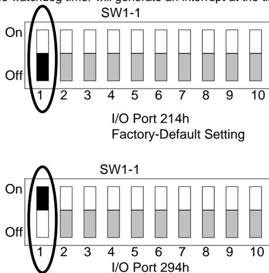
Figure 5-1 SW1-1: Watchdog I/O Port Address Select
