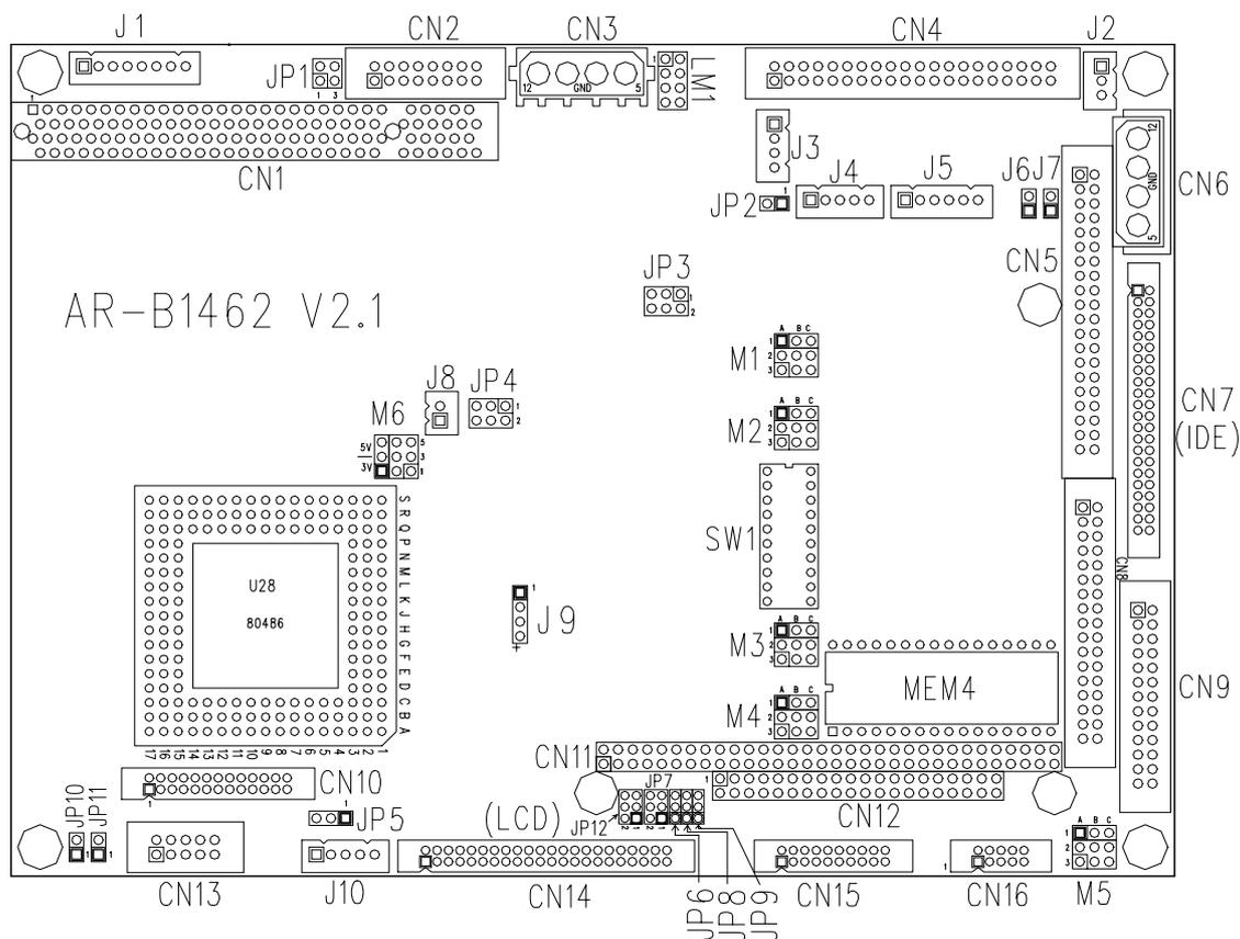
Figure 3-1 AR-B1462 Jumpers & Connectors Placement
