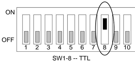
**Figure 3-13 SW1-8: COM-A RS-232/TTL Select**
