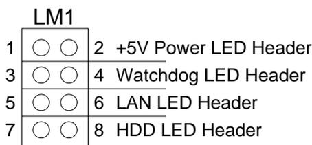
Figure 3-10 LM1: LED Header
