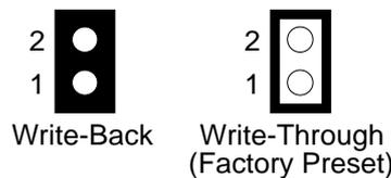
Figure 3-36 JP10: Write-Through/Write-Back CPU Select
