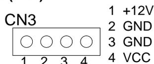
Figure 3-33 CN3: CPU Cooling Fan Power Connector
