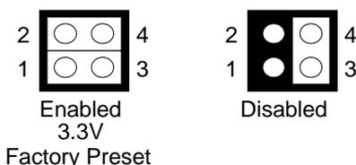
Figure 3-34 JP1: PCI Connector Power Select
