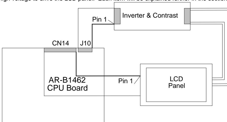
Figure 4-3 LCD Panel Cable Installation Diagram
