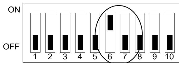
Figure 6-6 5V Large FLASH (29FXXX) Switch Setting
