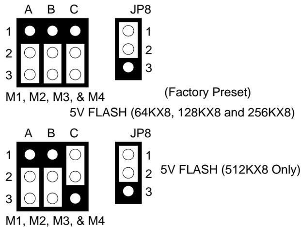
Figure 6-9 5V FLASH (29CXXX & 28EEXXX) Jumper Setting
