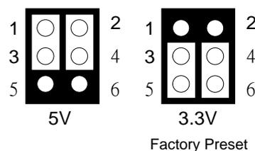
**(6) LCD Panel Display Connector (CN14)**
