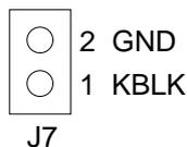
Figure 3-19 J7: Keyboard Lock Header
