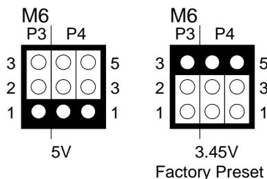
Figure 3-30 M6: CPU Logic Core Voltage
