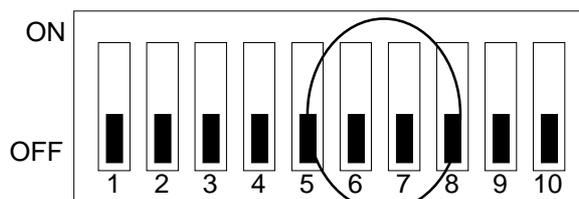
Figure 6-4 UV EPROM (27CXXX) Switch Setting
