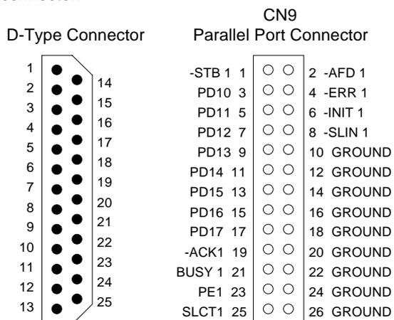
Figure 3-5 CN9: Parallel Port Connector
