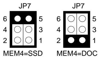
**Figure 6-11 JP7: Disk On Chip Memory Address Setting**
