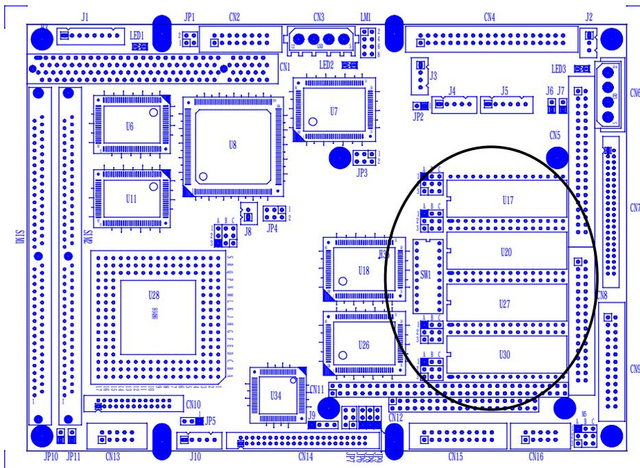
Figure 6-1 Switch & SSD Type Jumper Location
