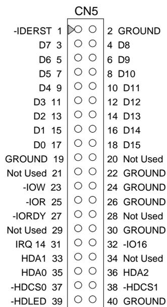
Figure 3-3 CN5: Hard Disk (IDE) Connector
