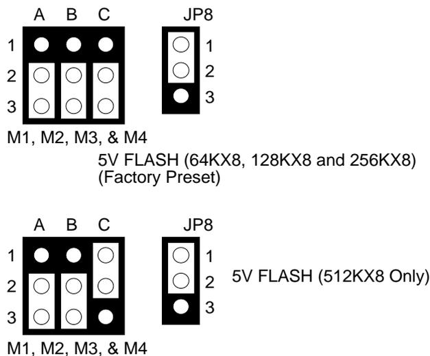
Figure 6-7 Large Page 5V FLASH Jumper Setting
