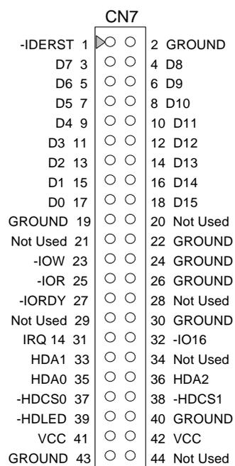
Figure 3-4 CN7: Hard Disk (IDE) Connector
