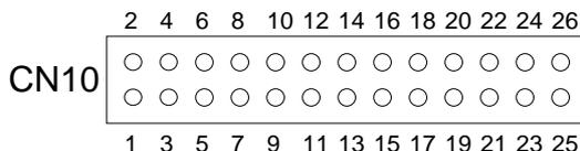
Figure 3-29 CN10: 26-Pin Audio Connector
