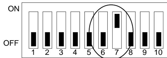
Figure 6-8 5V FLASH (29CXXX & 28EEXXX) Switch Setting
