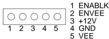
Figure 4-6 J10: LCD Control Connector
