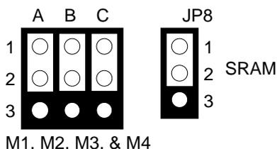
Figure 6-10 SRAM Jumpers Setting
