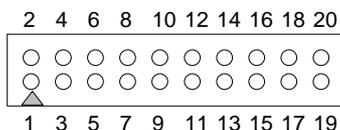
**Figure 3-16 CN15: RS-485/RS-422 Connector**
